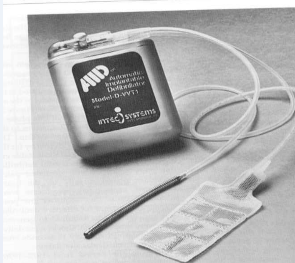
Fig. 3. First clinical model of the implantable cardioverter-defibrillator (ICD) shown with superior vena cava catheter and patch electrode.
